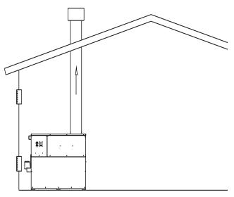
FIG. 7 Outside Combustion Air - Two Openings
